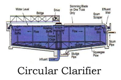
The **Skimming Zone** is at the surface of the tank. Solids and greases that have a specific gravity of less than 1.0 will float to the surface of the clarifier. A skimmer arm is attached to the rake assembly. It skims the surface as the rake rotates. In a rectangular tank the sludge rakes act as skimmers when the chain brings them to the surface. Floating scum is deposited in a grease or scum hopper. This grease and scum must be properly landfilled to prevent odor problems.
